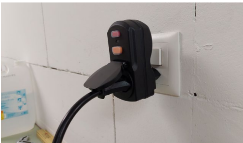
Figure 4: RCD mobile de 30 mA (source: Electrosuisse)
